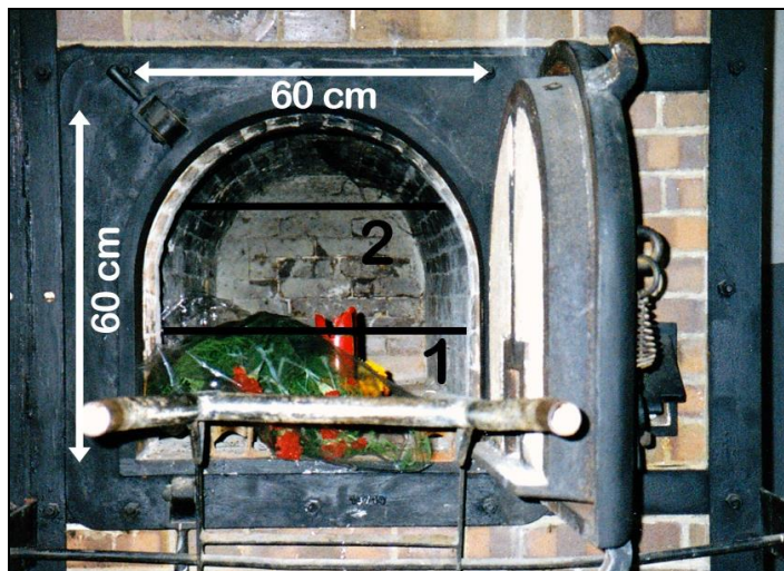
Illustration 36: Coke-fired double-muffle furnace by the Topf Company in the Mauthausen Concentration Camp with identical muffles to those that were installed in Auschwitz. The two horizontal lines represent the height of two corpses on top of each other on the muffle grate (Mattogno 2019, p. 650).
