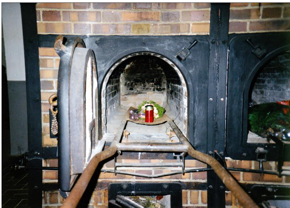
Document 11: Corpse-introduction stretcher in the left muffle of the double-muffle Topf Furnace at CC Mauthausen. Mattogno/Deana, Part 3, Photo 84, p. 68.
