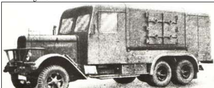
Illustration 25: Sd.-Kfz. 93, clothing decontamination vehicle, Henschel 33G1 (picture from Milsom 1975, p. 145)
