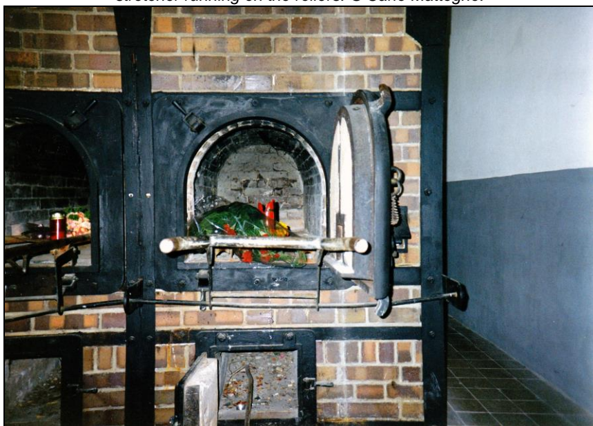
Document 43: Crematorium of Mauthausen. Topf coke-fired double-muffle furnace, Auschwitz Type. Loading system of furnace: fixation shaft, mobile roller system, and corpse stretcher. Front view. © Carlo Mattogno.
