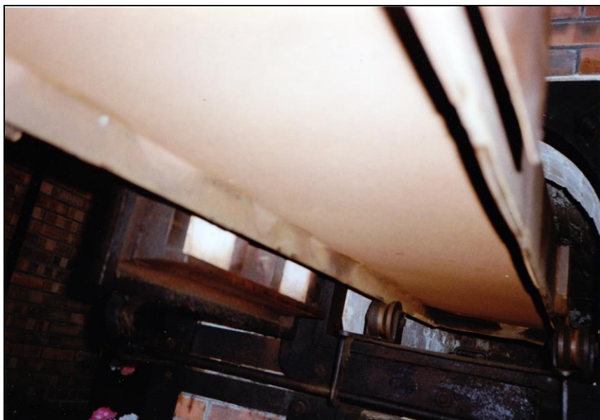
Document 42: Crematorium of Buchenwald. Topf triple-muffle coke-fired furnace. Central muffle. Corpse-introduction cart. Lower side. Rims of the stretcher running on the rollers. © Carlo Mattogno.
